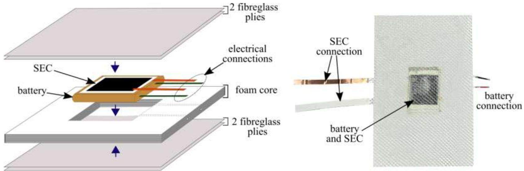
The composite was fabricated using the hand-lay method and allowed to cure for at least 24 hours before any testing.
