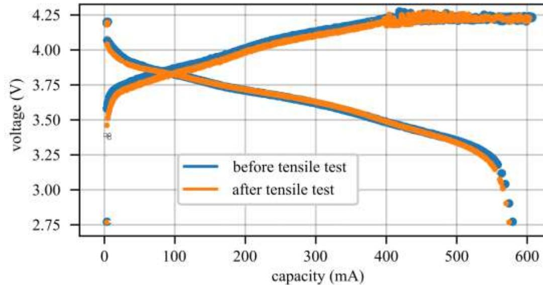
Little change in battery's performance after tensile test showing slight decrease in electrochemical efficiency
