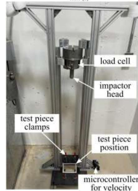
drop weight impact test machine
