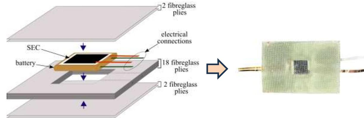
Laminate with embedded SEC and battery
