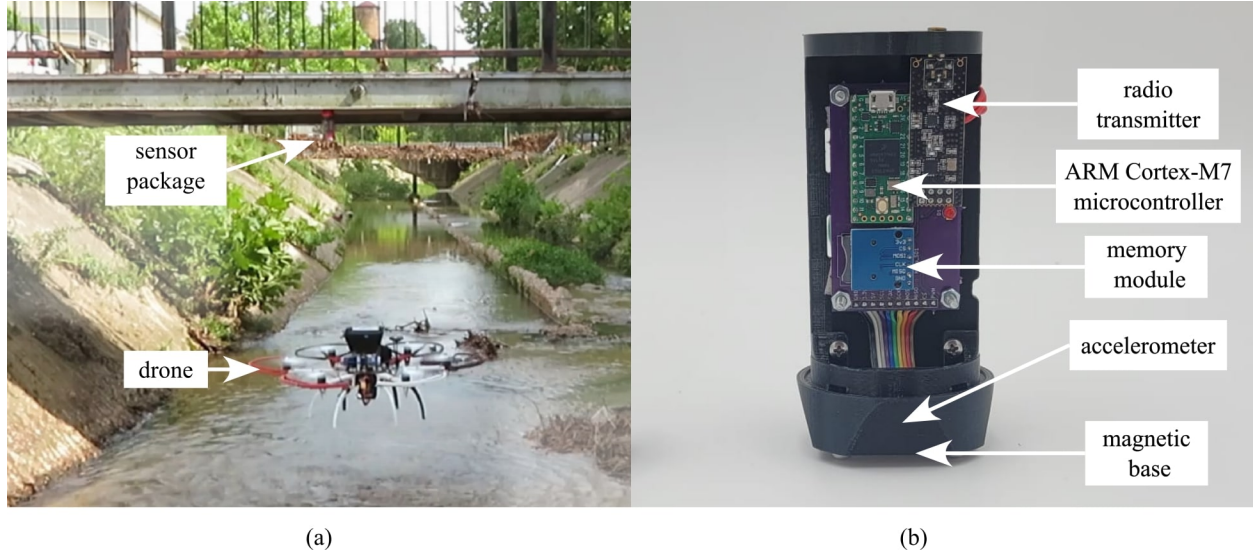
Figure 2. The drone-deployable sensor package with (a) a field deployment; and (b) key components annotated.
