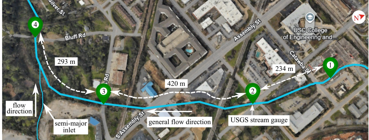
Figure 2. Map view of Rocky Branch creek showing green location markers representing the position of the deployed sensor nodes and the distances between them, starting from number one (upstream) to number four (downstream). Base imagery from Google Earth, © Google; Accessed: Dec 15, 2025.
