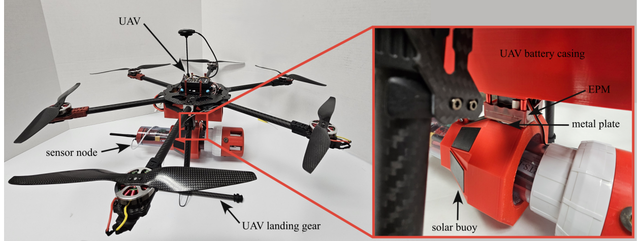
Figure 4. Sensor node docked under a hexacopter UAV with EPM-based deployment mechanism shown on the right.
