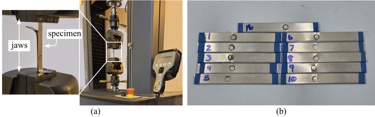
Figure 3: Testing configuration, showing: (a) the MTS Exceed E43 tensile tester in use; and; (b) all test specimens.
