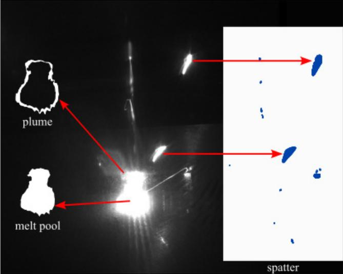
Figure 4. The extracted melt pool, plume, and spatter from the printing image.
