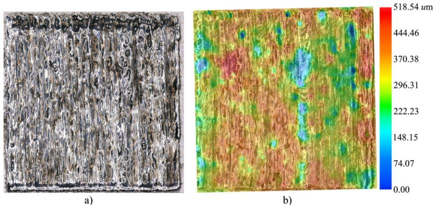
Figure 2. The sample in the research: a) the last layer's surface quality and b) the printed specimen surface height.
