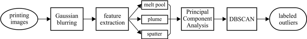
Figure 3. Flowchart for in-situ monitoring and unsupervised clustering analysis in laser powder bed fusion.
