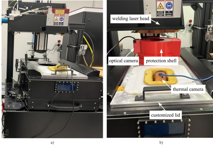
Figure 1. Experimental data collection setup on the metal 3D printer: a) the printer with the customized cover and b) data collection setup with the optical and thermal cameras.
