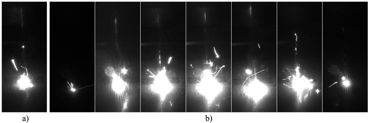
Figure 6. The clustering frames from unsupervised learning DBSCAN: a) the normal printing frame and b) seven outliers from the DBSCAN.
