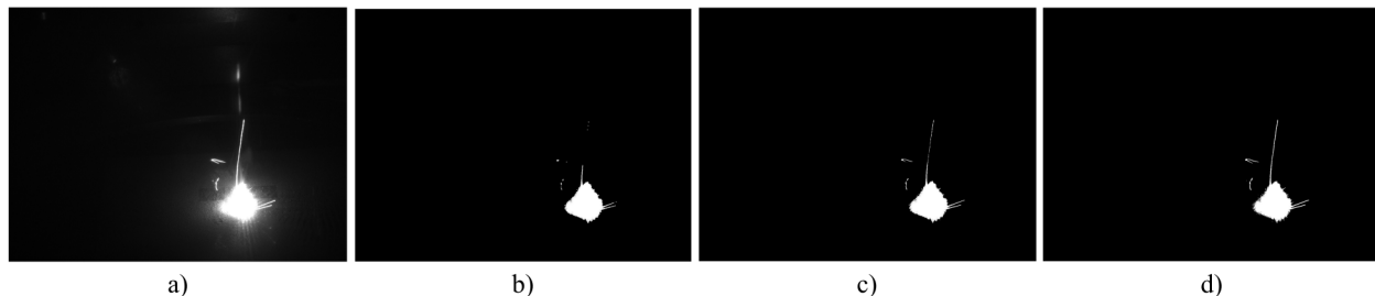
Figure 4. Splatter image processing showing: a) the raw splatter image; b) splatter with Gaussian blur, erode, dilate, and threshold filter; c) splatter with Gaussian blur and threshold filter; and d) splatter with threshold-only filter.
