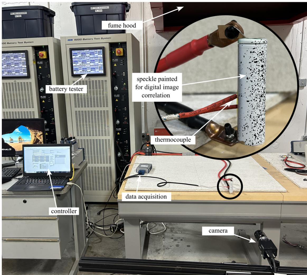
Figure 2. Battery testing setup showing the battery testers connected to a single 18650 cell under a high-C (40-A) discharge.
