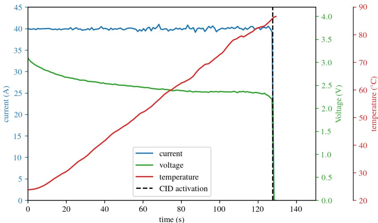
Figure 3. Experimental Electrical and Temperature response of 40-amp discharge.
