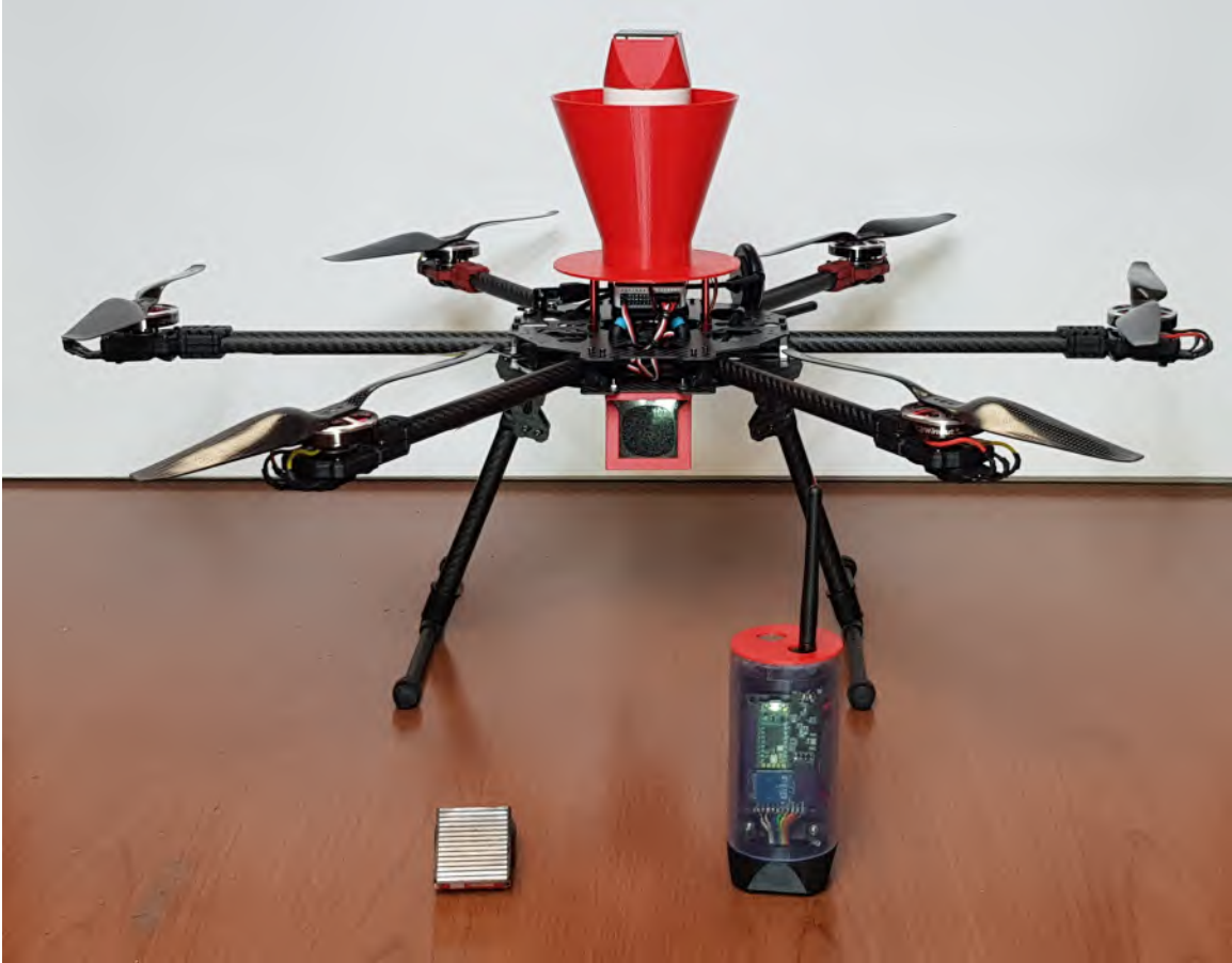
Figure 1.2: Various components of the rapid structural health monitoring system.
