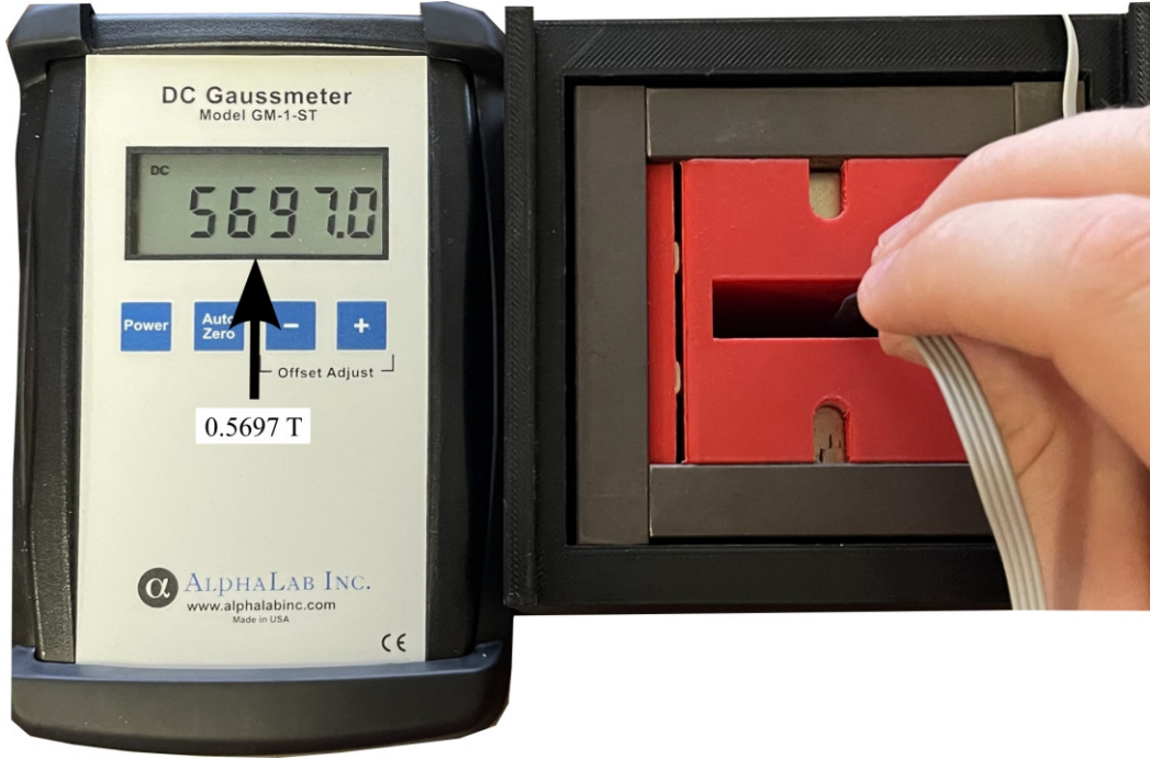
Figure 2.13: Recording magnet inductance using a Gaussmeter.
