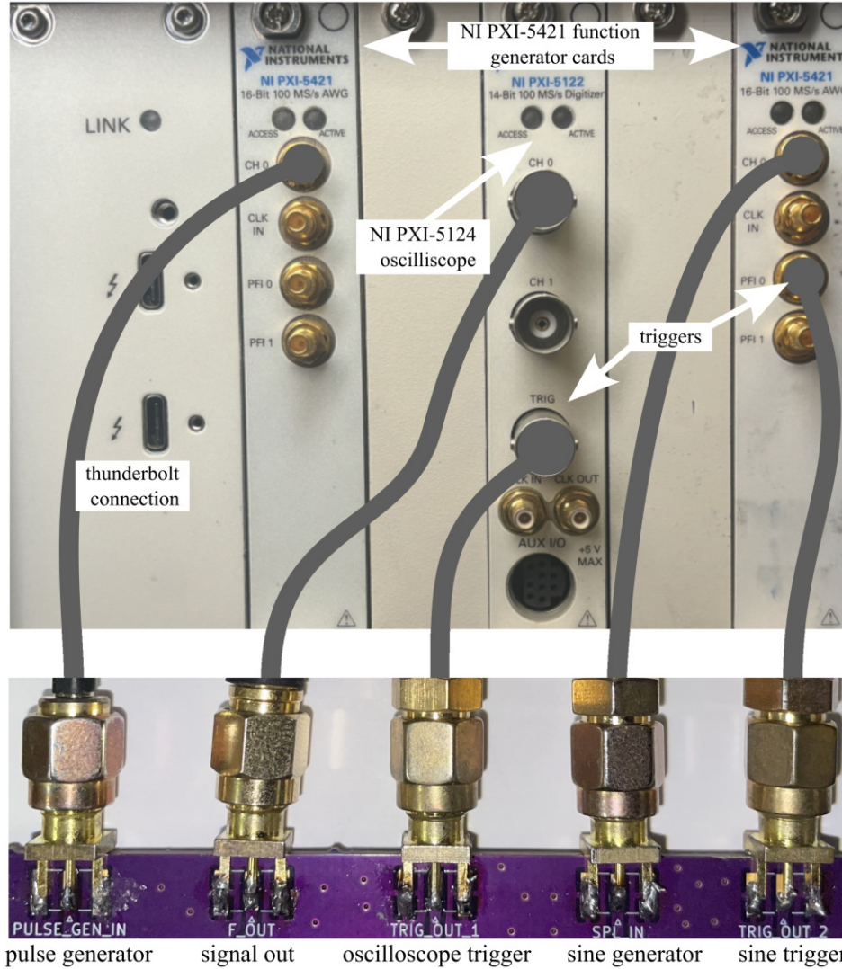
Figure 2.18: Wiring diagram from the PXI cards to the control board.
