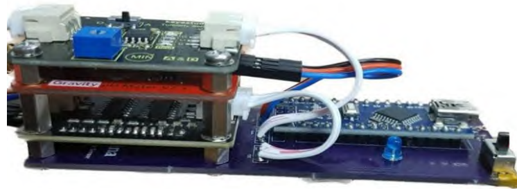
Figure 2.13: Compact PCB integrating the electronic components for the in-situ water quality sensor package.
