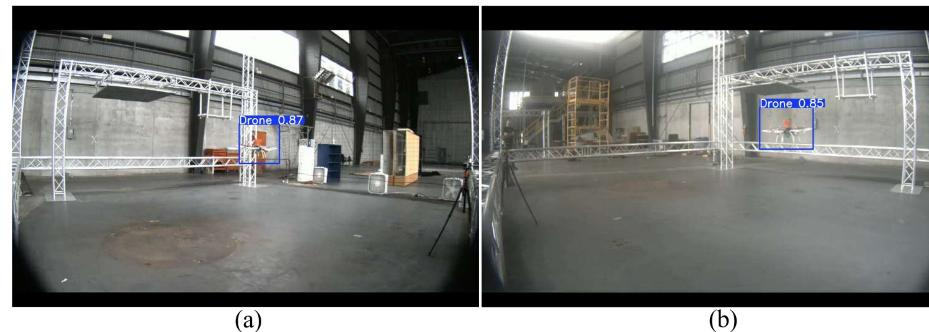
Camera views, showing: (a) the left camera view, and; (b) the right camera view with YOLO bounding box confidence levels.
