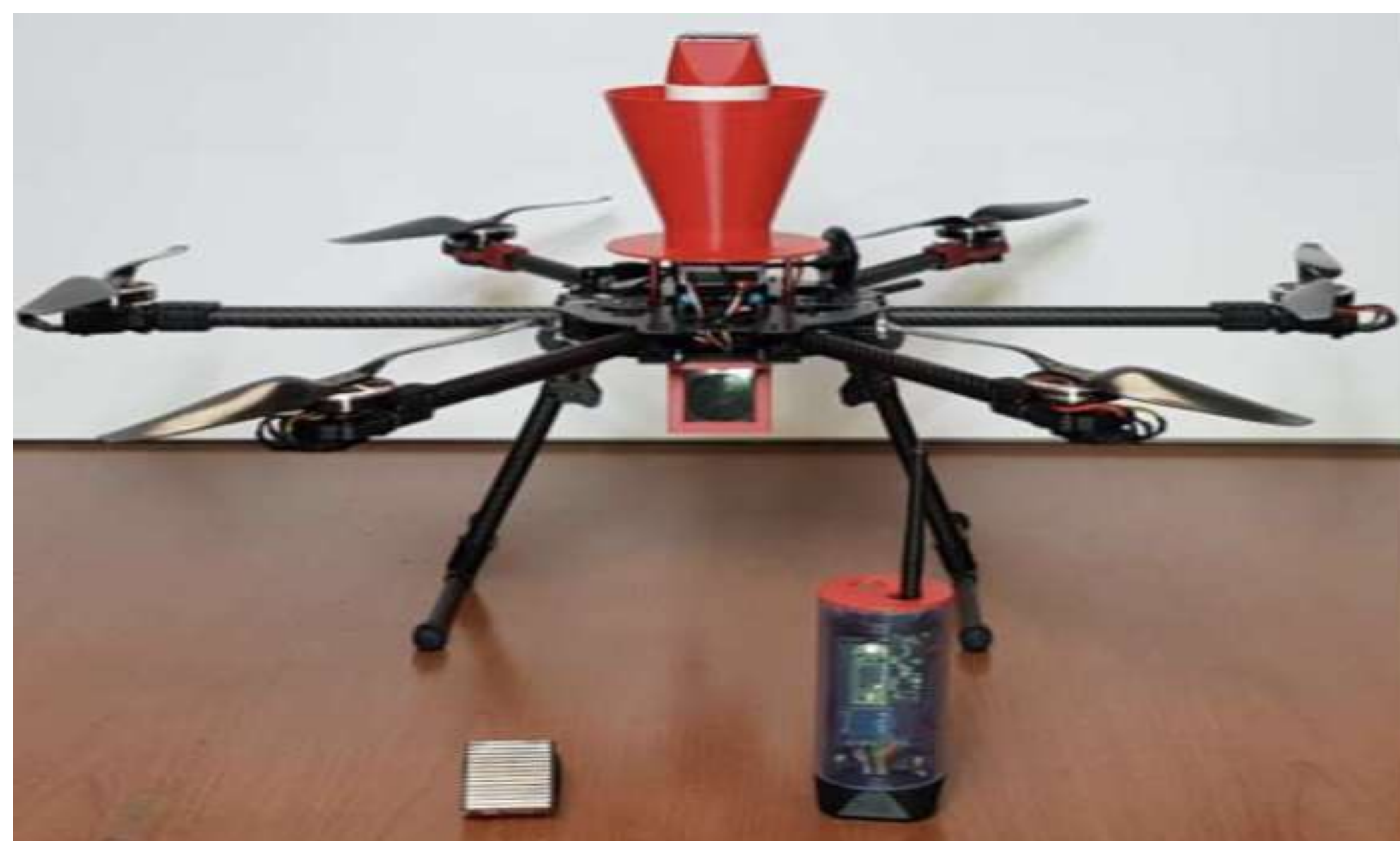
Image shows UAV used for sensor deployment and sensor package used for data collection.
