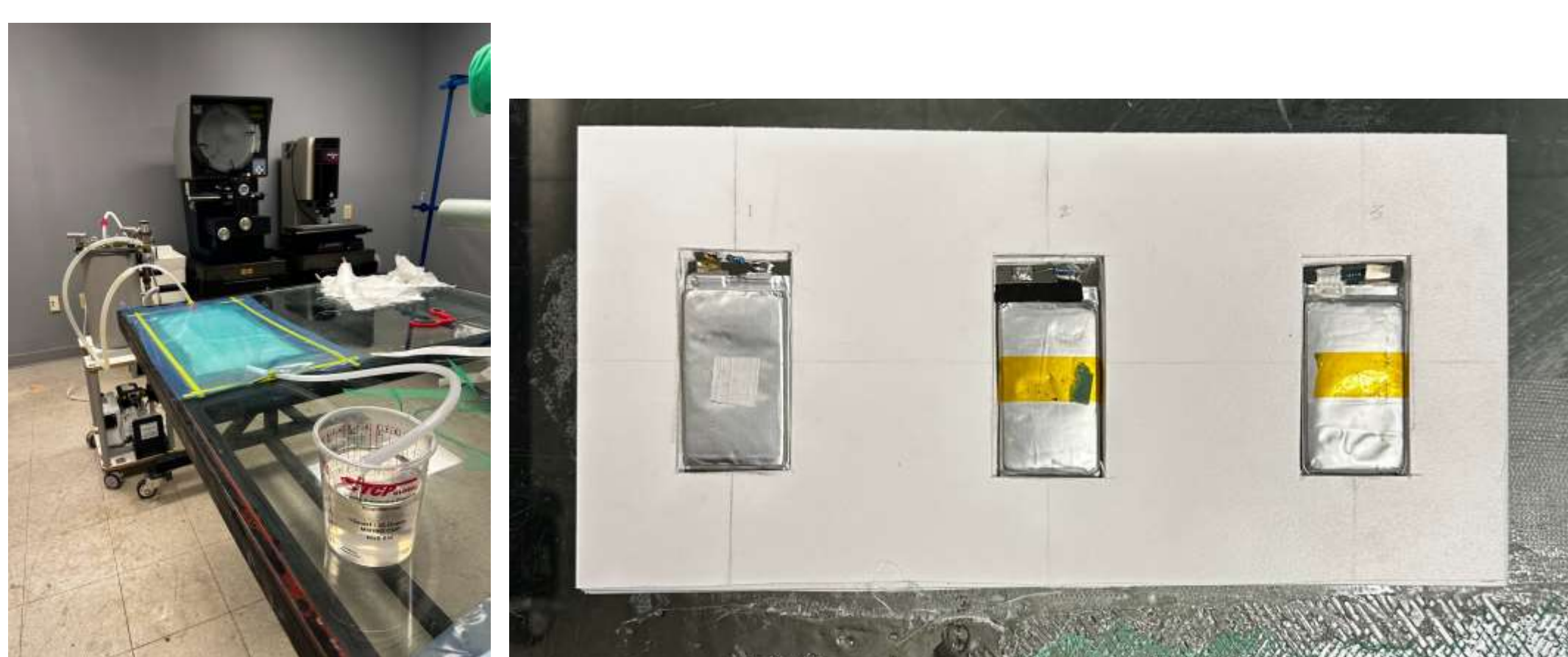
Fig. 2. VARTM setup (left) and a structural battery layout (right).
