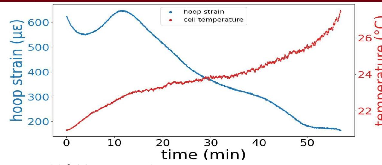
30Q005 cycle 50 discharge strain and temp data.
