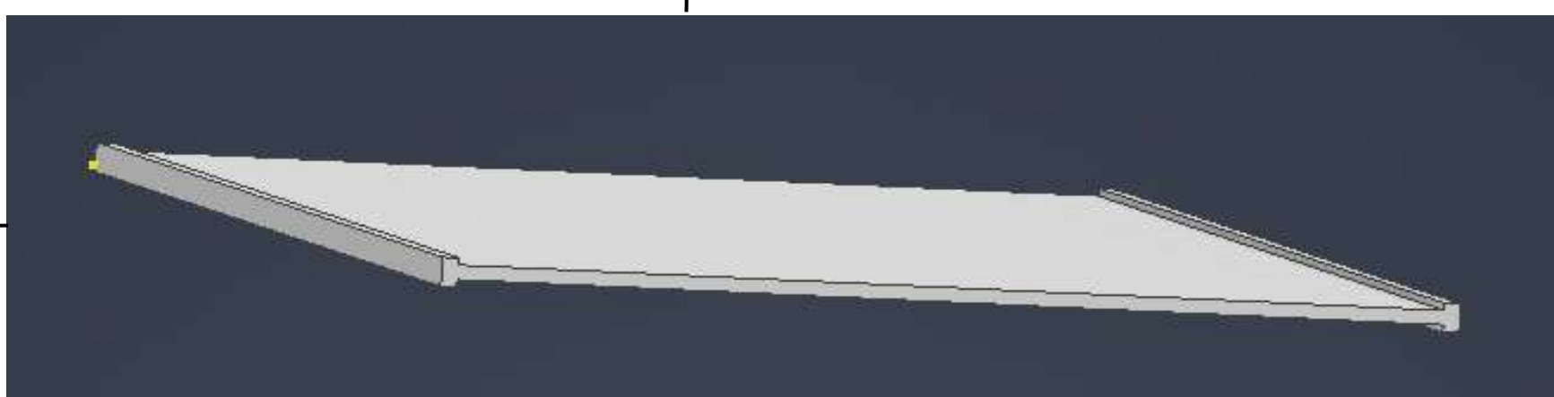
Figure 2. Upper platform designed to slide along the rails of the avionics box
