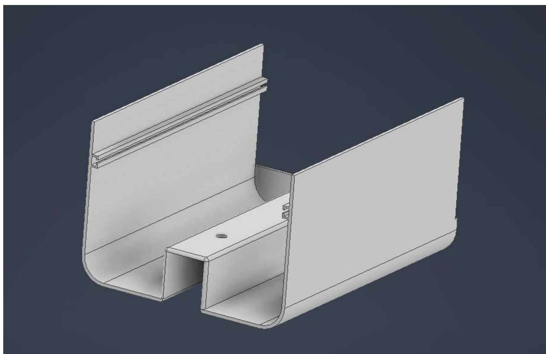
Figure 1. Avionics bay depicting lower slots for holstering batteries and rails for upper platform.
