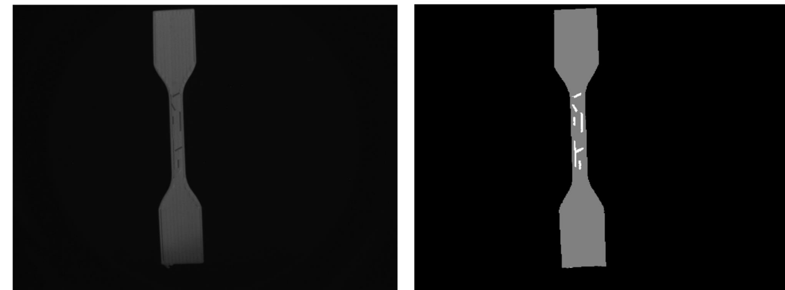
Image segmentation-based defect detection with the U-Net convolutional neural network.
