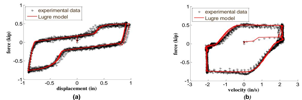
Figure 6: Model fitting of the MFD: (a) force-displacement loop; and (b) force-velocity loop
