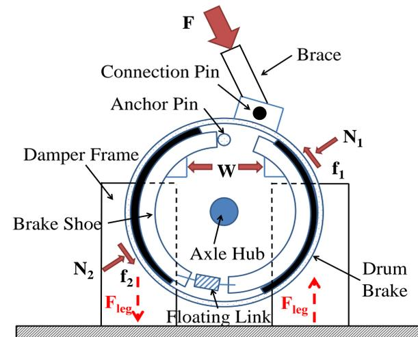
Figure 2: Schematic of the braking mechanism in the MFD
