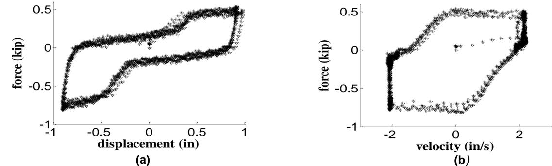
Figure 4: Dynamic of the MFD under hydraulic pressure of 1500 psi: (a) force-displacement plot; and (b) force-velocity plot.
