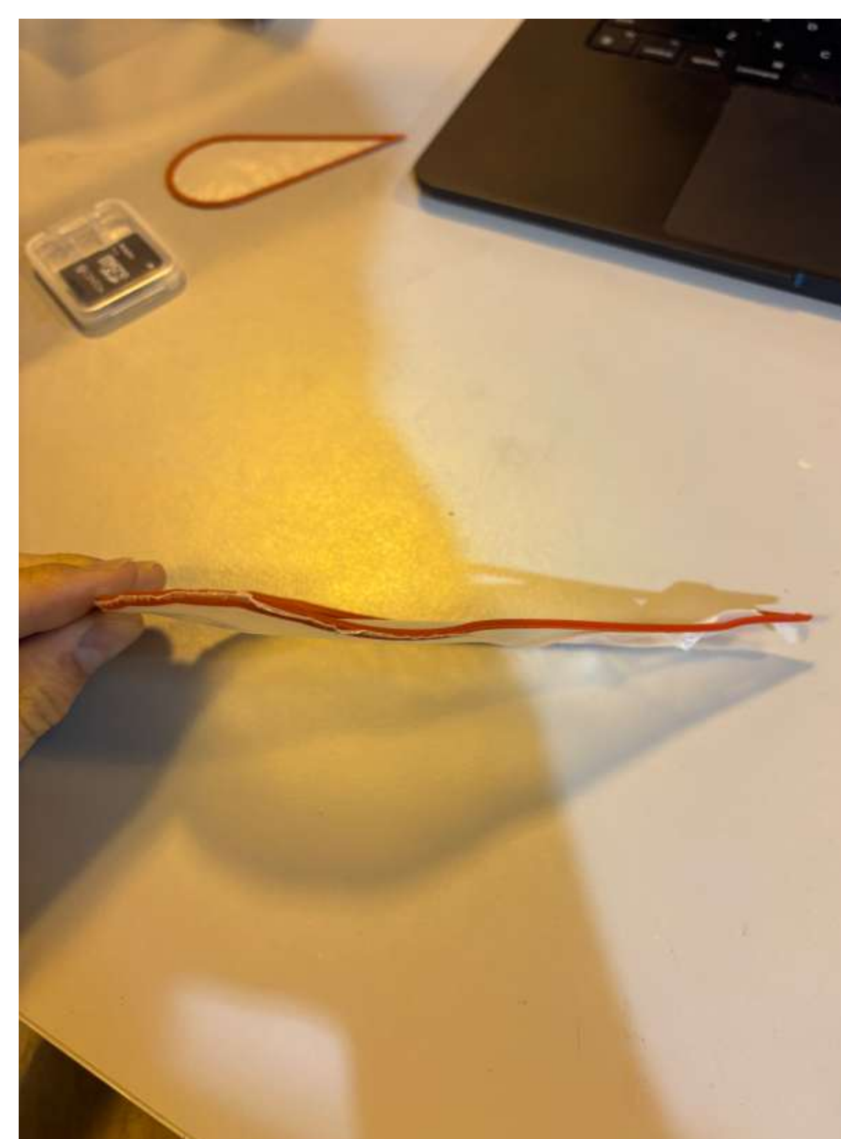
Initial tear drop shape design with melted wing frame, causing frame deformities and wax paper detachment
