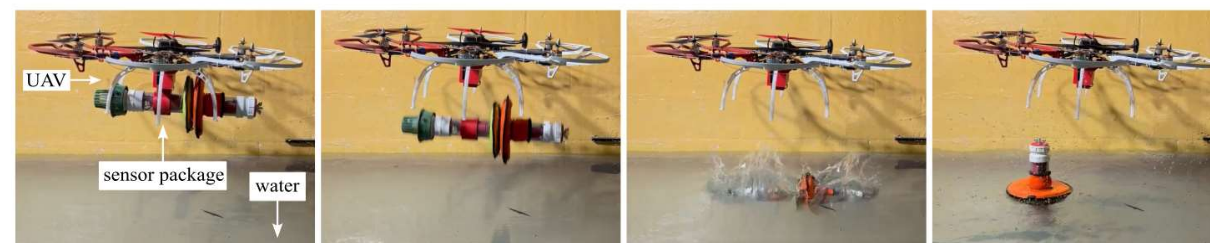
Figure 2: UAV deployment of the In-situ water quality sensor node
