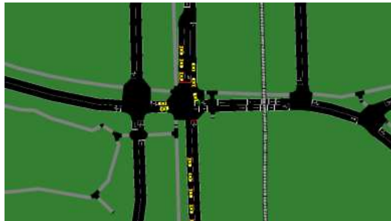
SUMO network (Buist/Spruill Intersection)
