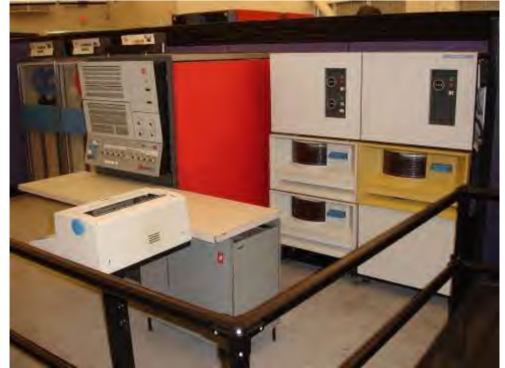
IBM System/360 Model 30 CPU (red, middle of picture), tape drives to its left, and disk drives to its right, at the Computer History Museum
