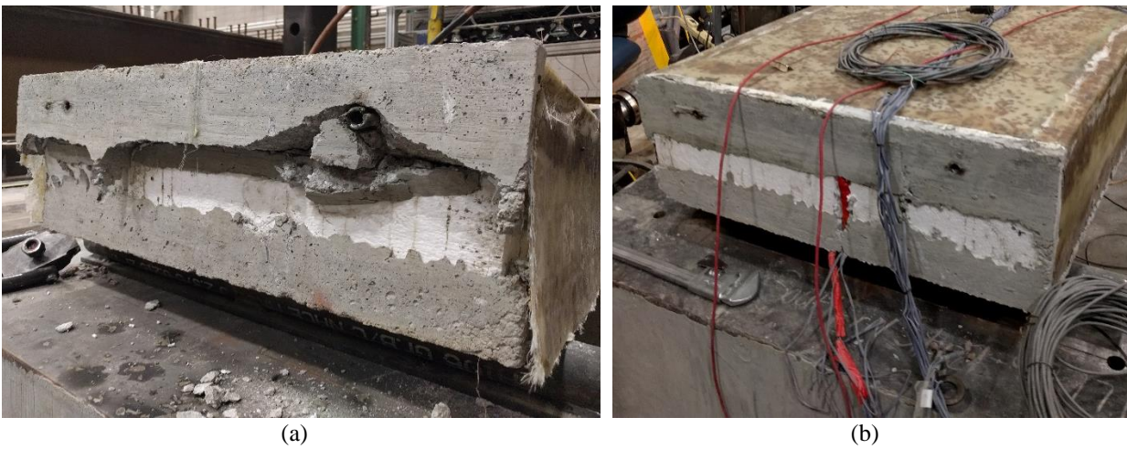
Figure 22 (a) Slip at the end of the south side, (b) No slip is detected at the north side
