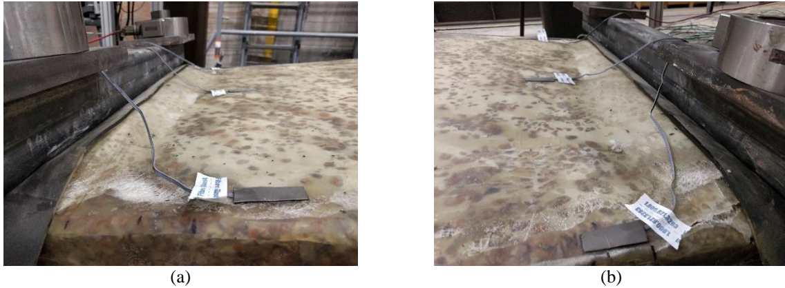
Figure 25 Wrinkling of the top FRP, (a) view for east side and from the (b) west side
