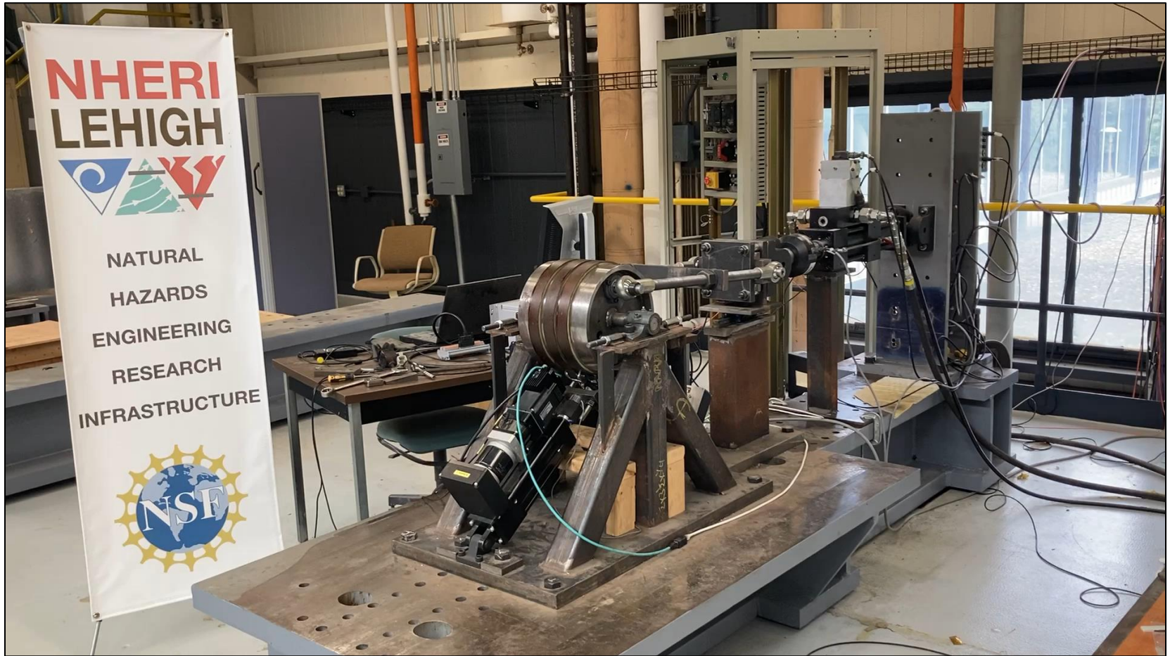
Vid. 1. BRFD passive mode operation.
