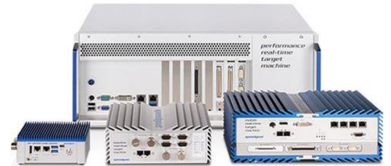
Speedgoat Systems for programming FPGAs in MATLAB/Simulink
