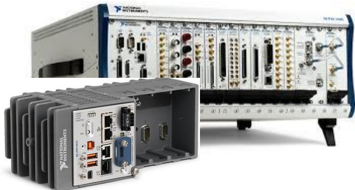
NI systems for programming FPGA in LabVIEW
