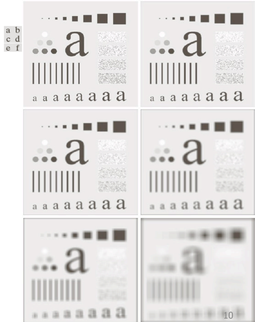
FIGURE 3.33 (a) Original image, of size 500 \times 500 pixels. (b)–(f) Results of smoothing with square averaging filter masks of sizes m = 3, 5, 9, 15, and 35 , respectively. The black squares at the top are of sizes 3, 5, 9, 15, 25, 35, 45, and 55 pixels, respectively; their borders are 25 pixels apart. The letters at the bottom range in size from 10 to 24 points, in increments of 2 points; the large letter at the top is 60 points. The vertical bars are 5 pixels wide and 100 pixels high; their separation is 20 pixels. The diameter of the circles is 25 pixels, and their borders are 15 pixels apart; their intensity levels range from 0\% to 100\% black in increments of 20\% . The background of the image is 10\% black. The noisy rectangles are of size 50 \times 120 pixels.
