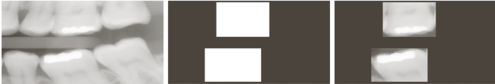
FIGURE 2.30 (a) Digital dental X-ray image. (b) ROI mask for isolating teeth with fillings (white corresponds to 1 and black corresponds to 0). (c) Product of (a) and (b).
