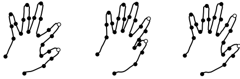
Fig. 2 Three example 2D shape contours of the human hand. Each contour has 24 landmarks, where one white landmark corresponds the tip of the thumb and the other white landmark corresponds the tip of the index finger
